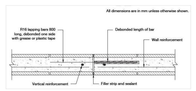
NZS 4229 Figure 12.2 – Control joint detail for solid-filled walls and partially filled walls where horizontal bars are placed between floors but not bond beams
