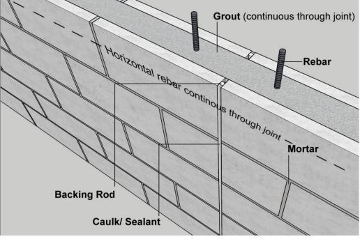
Control joint example, at bond beam level
