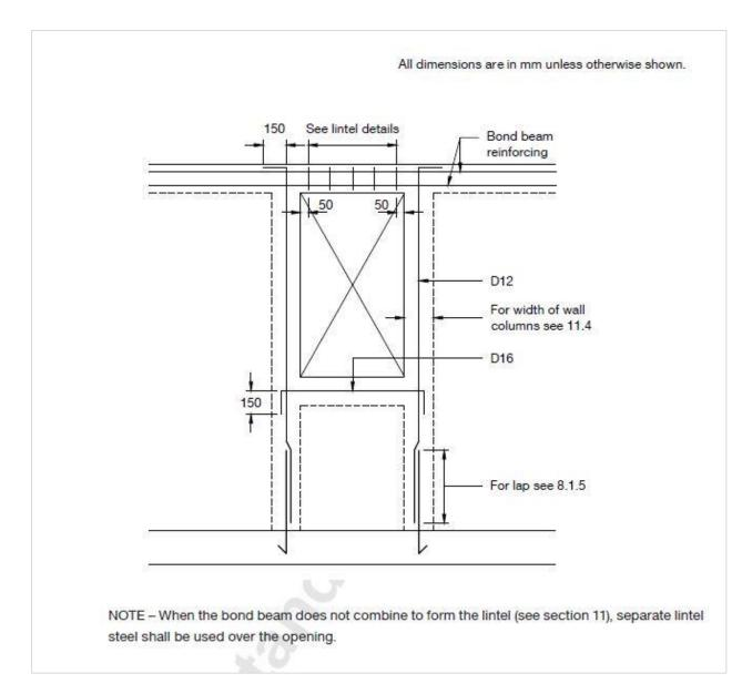
NZS 4229 Figure 8.1 – Reinforcement above and below openings
