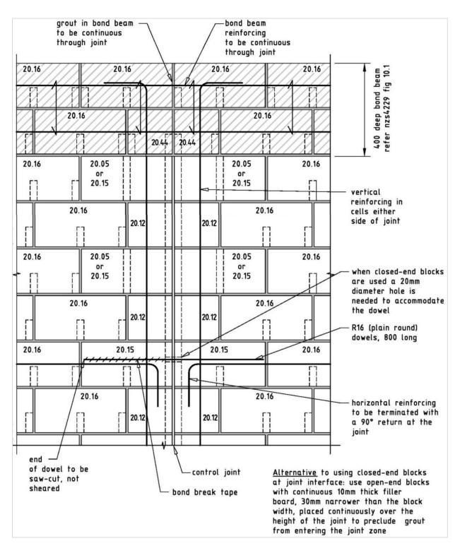
CMM, Figure 3 – Control joint elevation
